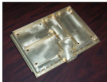
Fig. 4. This conduction-cooled, aluminum-encapsulated highly oriented pyrolytic graphite VME format aircraft power supply housing dissipates 235 W. (Courtesy of k Technology Corp.)
