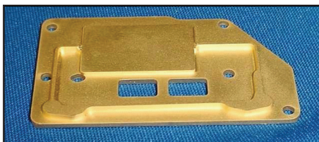
Fig. 5. This thermoelectric cooler base uses Al/SiC-encapsulated highly oriented pyrolytic graphite (HOPG), which can have greater thermal conductivity than Al/SiC while maintaining its approximate CTE. (Courtesy of Ceramics Process Systems.)
